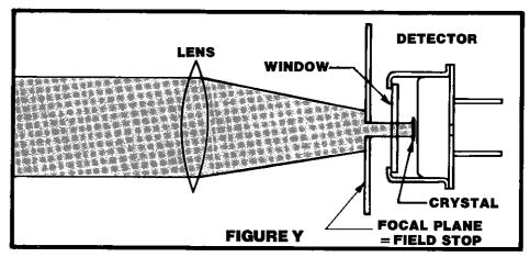
ter limiting the optical system's angular field of view.
